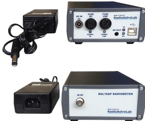
FIGURE 2.9: The RAL10AP receiver: you can see (on the top) the socket for the mains power supply to 12 VDC, the fuse holder with interruption indicated via led for the main power supply and the external unit power supply through the coaxial cable (leds turn off when the respective fuse is burnt out), the audio output of post-detection ( BF-OUT ) and the USB port for the connection to your PC (the leds indicate the flow of data). On the rear panel (below) is the F connector for the signal input ( IN RF ) coming from the external unit.
